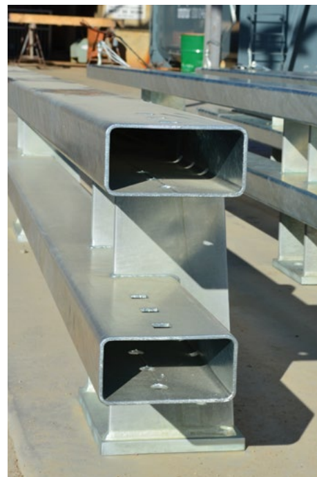
Figure 1: With a specified minimum HDG coating thickness of 85 µm, AS/NZS 2312.2 can be used to estimate this bridge rail will be protected from rust for over 50 years in a C3 (medium) environment.
