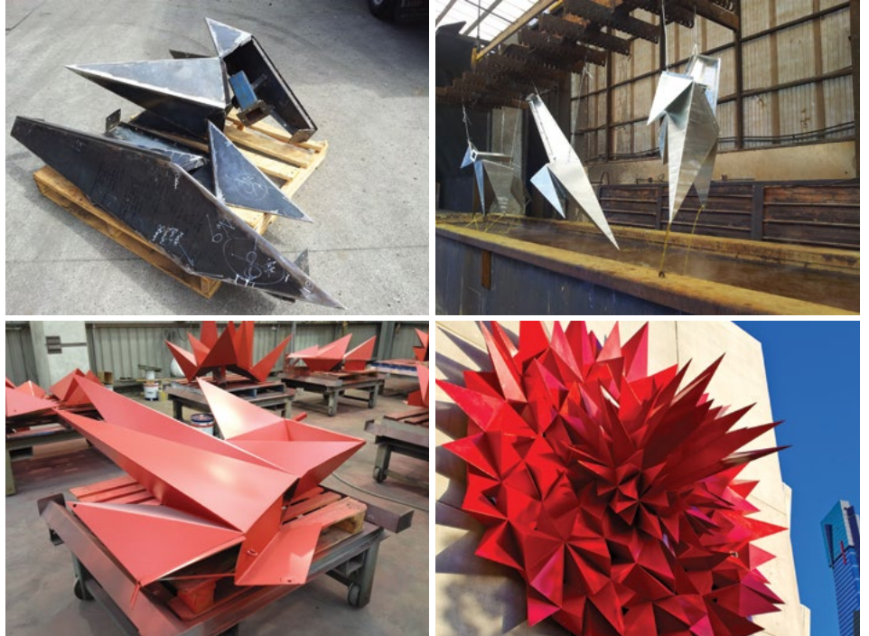
Figure 4: The Moment by Damian Vick, showing the four key stages of fabrication, galvanizing, painting, and the final structure in place. This aesthetic sculpture is an example of a complex shape with sharp edges and is therefore perfectly suited to a duplex coating.
