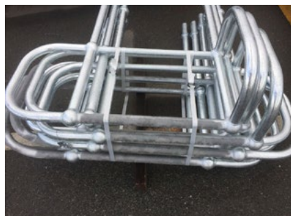
Figure 14: Dull appearance on one section of the a fabricated handrail
