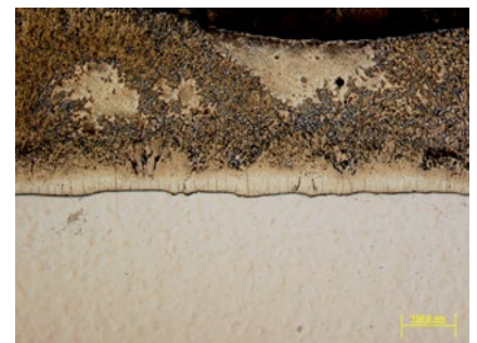
Figure 13: Micrograph showing part of the structure of a part dull, part shiny galvanized coating
