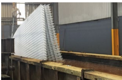
Bundles of galvanized reinforcement mesh being removed from the quench bath
