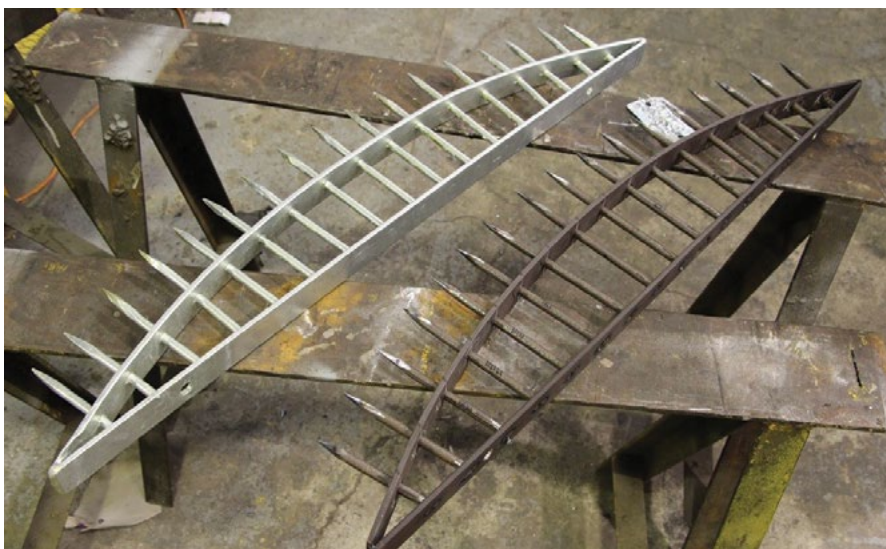
Figure 13: Restoration for Sydney Water of an old spike guard was successfully completed using GMA braze welding
