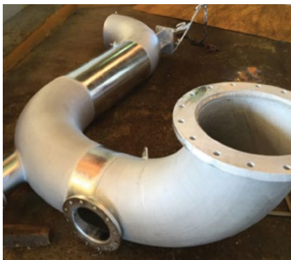
Figure 10: Another example of steels of widely different chemical composition causing an initial appearance issue for the customer. In most cases this affect is aesthetic and there is usually no detrimental effect to the durability of the article
