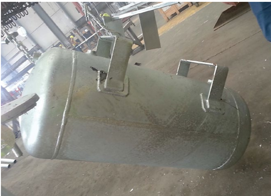
Figure 8: Blowout from undersized hole for venting the overlapping area of the plate fully welded to the large hollow vessel
