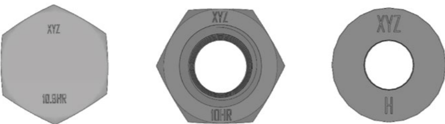
Figure 12: Marking for class 10.9 High strength bolts, nuts and washers
