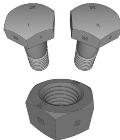
Figure 9: Marking For Tower Bolts And Nuts
