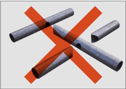
Figure 17: Internal Vent Holes with No Inspection Holes – Not acceptable
