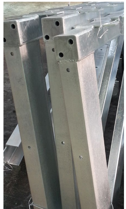
Figure 14: Closed Hollow Sections – Unsatisfactory
