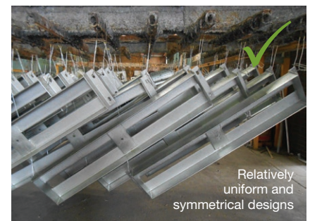
Figure 5: Avoid Distortion with Good Design
