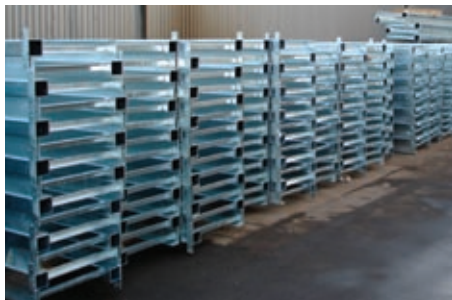
Galvanized pallet shelving before fitting of corrugated iron.
