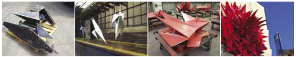
Figure 3: The Moment by Damian Vick, showing the four key stages of fabrication, galvanizing, painting and the final structure in place. This aesthetic sculpture is an example of a complex shape with sharp edges and is therefore suited to a duplex coating.
