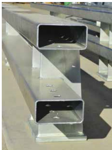
Figure 1: With a specified minimum HDG coating thickness of 85µm, AS/NZS 2312.2 can be used to estimate this bridge rail will be protected from rust for over 50 years in a C3 (medium) environment.
